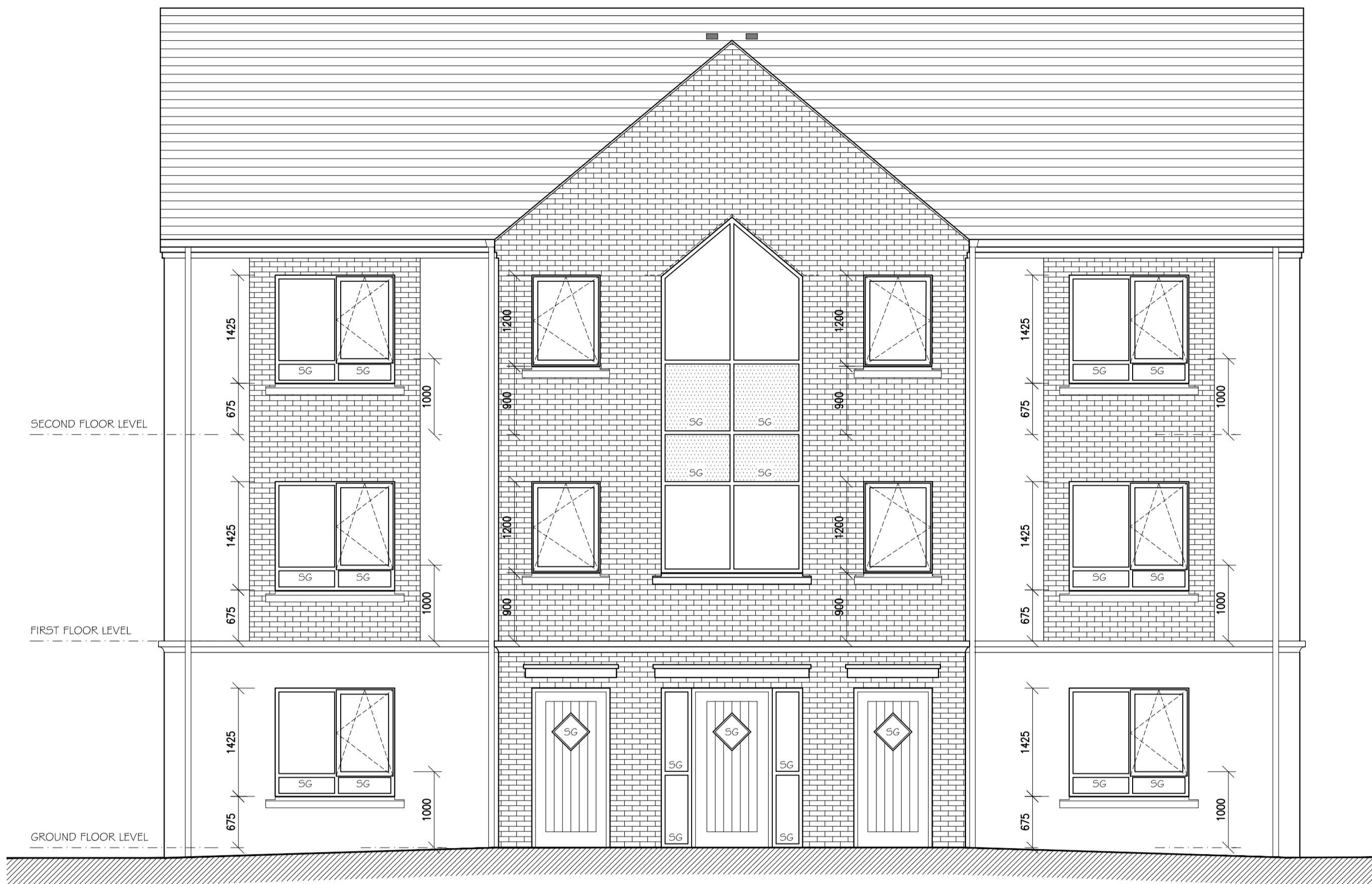
FRONT ELEVATION - APARTMENT BLOCK
